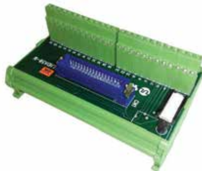
50 Pin Honda Connector Module for Robots
