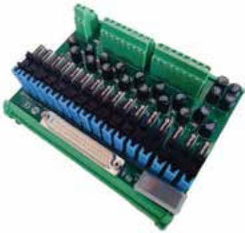
16 Channel DI Slim relay module with miniature fuse
