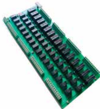
Customized Relay logic board
