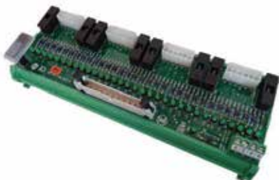
32 channel DI module with Molex connector
